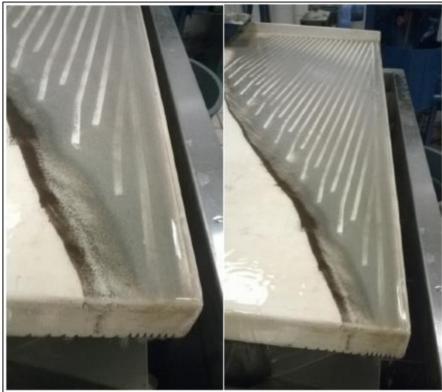
Figure 13.3 Picture of a 200 Micron Gravity Separation Test
