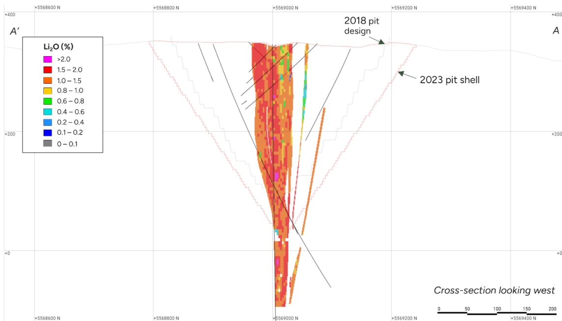
Figure 2: Cross Section Showing 2023 Resource Pit Shell, 2018 PEA Pit Design, and 2023 Block Grades
