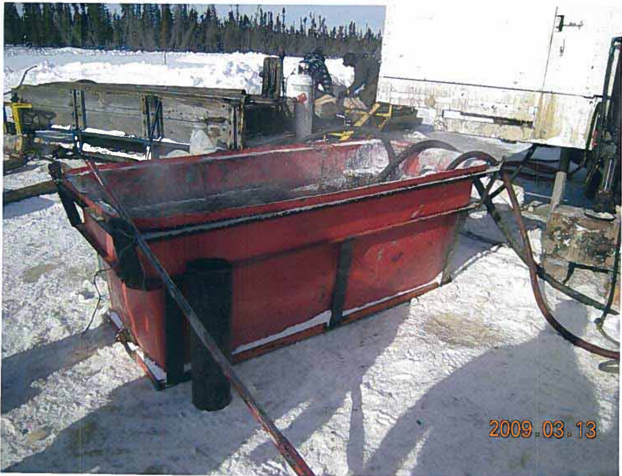
MV2007C0039 - Avalon Ventures Ltd. Tub for the collection of drill cuttings/water at the Foraco drill.
